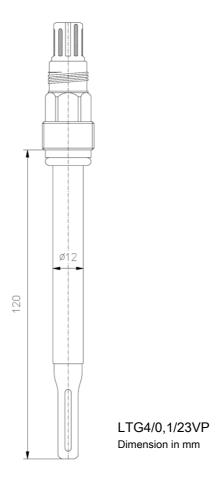
The conductivity measuring cell LTG4/0.1/23 is a four-electrode measuring cell with a glass shaft, platinum-plated sheet electrodes and an integrated temperature sensor. A wide measuring range, robust design, low maintenance and easy cleaning characterize this measuring cell for universal use in water treatment, wastewater treatment, environmental and process technology.
